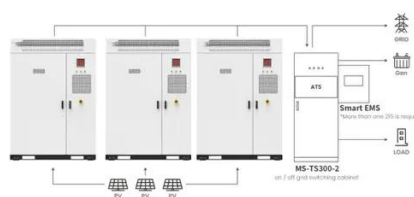
Application scenarios of energy storage battery products
